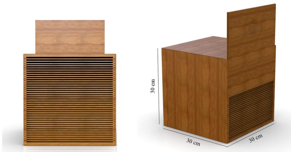
**Fig. 1** Front (left) and rear (right) views of a wooden trap designed for brown marmorated stink bug (*Halyomorpha halys*) overwintering adults. The trap is 30×30×30 cm in size with 4 mm between the layers inside, and a total of 35 layers. The wood material is pine plank. The layer material is plywood
