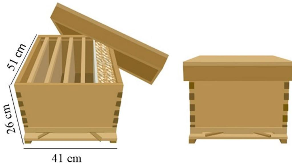
**Fig. 4** Opened (right) and front (left) view of a beehive box trap used in this study to trap brown marmorated stink bug (*Halyomorpha halys*) overwintering adults
