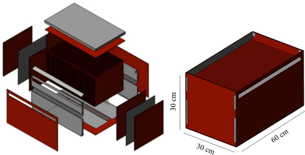
**Fig. 2** Assembled view (left) and internal view (right) of the black corflute trap used in this study to trap brown marmorated stink bug (*Halyomorpha halys*) overwintering adults
