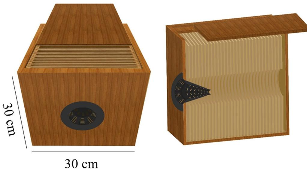
**Fig. 3** Front view (left) and profile view (right) of the wooden-made locked trap used in this study to trap brown marmorated stink bug (*Halyomorpha halys*) overwintering adults
